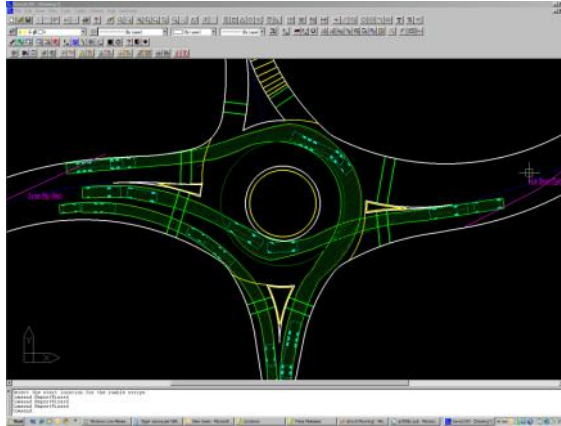
Use AutoTrack Roads Pro to add vehicles
